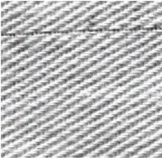
Figure 2. All width drill imperfection: thread pull off.
