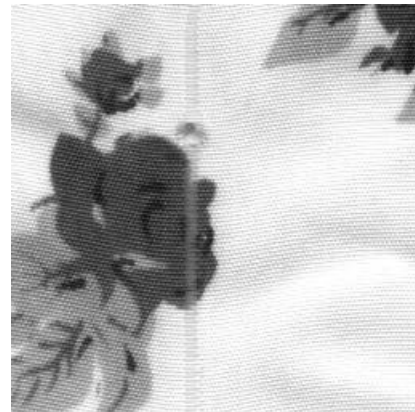
Figure 6. Defective colourful textile.
